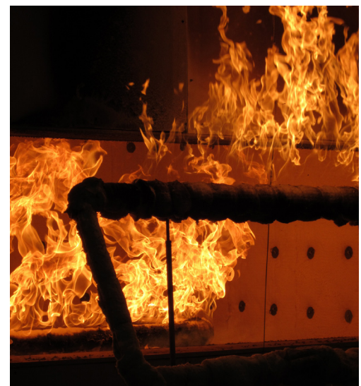
The International Building Code requires that walls with foam plastic insulation pass the NFPA 285 test. Image courtesy of Construction and Maintenance Solutions, LLC
